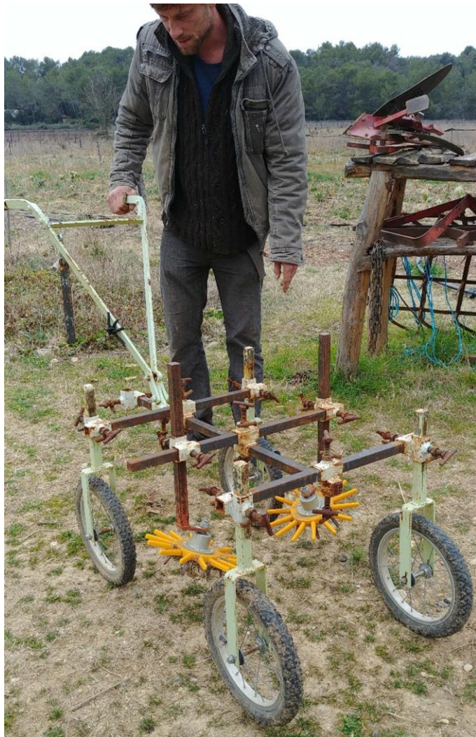
Figure 8: Outil multiusage auto-construit
